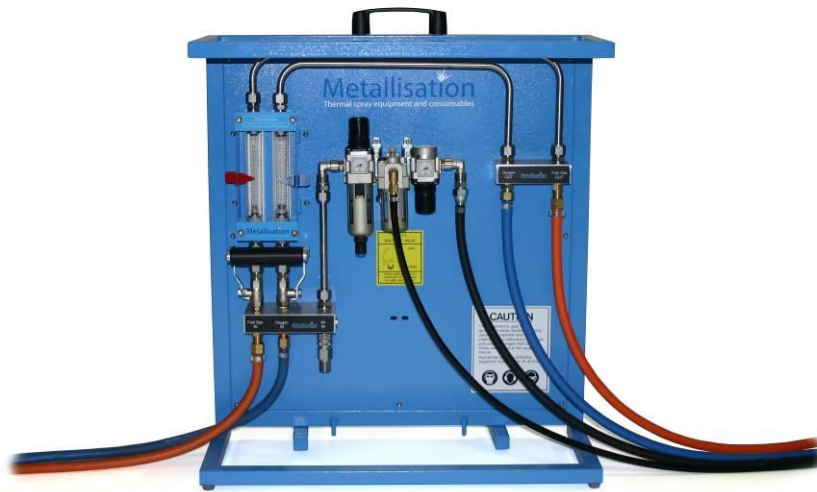
Supplies from regulators to flowmeters
